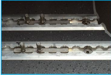
Place T-bolts in the rail. Two 35 mm pieces for the T-bolt in front of wheelarch and two 35 mm pieces behind the wheel case. Note that with the 35 mm T-bolt, the arrow with the letter F (front) faces the front of vehicle.
