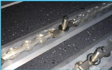
Place a washer over the wire ends of both front T-bolts before placing the chair.
