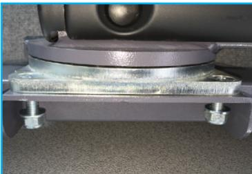
Mount the Smartseat Easy Tip & Fold on the single wheel arch bracket with 4 bolts, M10 x 35 quality, 10.9 or higher. Tighten bolts to 50 Nm. Mount the Tip & Fold Smartseats onto the wheelarch frame and secure using the provided bolts, washers, and locknuts, M10 x 35, grade 10.9 or higher. Tighten bolts to 50 Nm.
