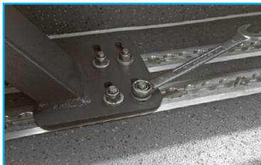
Place the second washer, followed by the self-locking M10 nut. Tighten nut to 50 Nm.
