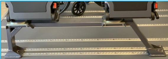
Place the bracket with the seat(s) on the T-bolt thread ends. Install the wheelarch frame onto the threaded studs of the T-bolts.
