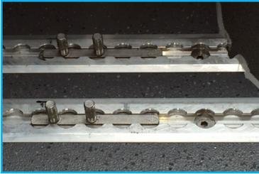
Place T-bolts in the rails onto the appropriate adjacent airline rails. Note that with the 35 mm T-bolts, the arrow with the letter F (front) always must face the front of vehicle.
