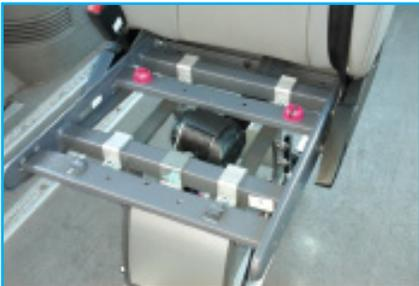
Mount the chair to the Smartlegs Legs using the mounting brackets and hex bolts. Quality 10.9 or higher nuts and bolts. First mount all nuts and bolts before securing them. Secure these bolts with a minimum torque of 20 Nm. There is no maximum limit to offset the seat LH or RH.
