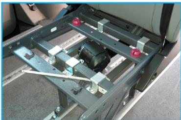
Mount the chair to the fixed legs using the mounting brackets and hex M8x45 nuts and bolts of quality 10.9 or higher. First mount all nuts and bolts before securing them. Secure these bolts with a minimum torque of 20 Nm.
