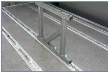
First place an underlay ring in the airline rail over the threaded rods of the foremost T-bolts. Then place the Fixed legs on the T-bolts.
