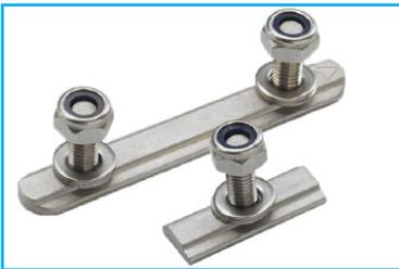
Place two T-bolts 76 mm and two single T-bolts. The single fitting comes to the front of the seatleg and the T-bolt 76 mm at the rear. Note that the arrow (with the letter F) must face the front of the vehicle.
