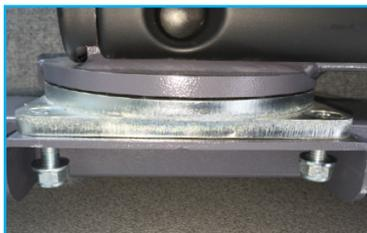
Mount the Smartseat Easy Tip & Fold on the single wheel arch bracket with 4 bolts, M10 X 35 quality, 10.9 or higher. Tighten bolts to 50 Nm.
