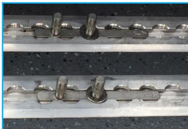
Place washer on one of the ends of both front T-bolts before the chair is placed. When the T-bolts are in the desired location, place one flat washer onto one of the threaded studs on each of the T-bolts.
