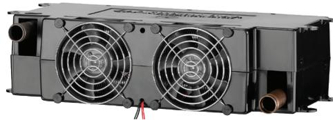
Compact Cozy Heat Exchangers (13.125" x 3.625" x 6.5") can be strategically placed to deliver heat to up to 3 different zones throughout the van. The exchangers can be installed either vertically or horizontally to easily integrate with interior configurations.
