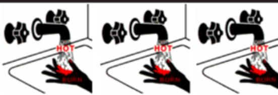
**Risk of Severe Burn or Death from Scalds.** Water temperature over 51°C (123.8°F) can cause severe burns instantly or death from scalds. See instruction manual before setting temperature at water heater. Feel water before bathing or showering. Temperature limiting valves are available, see manual.
